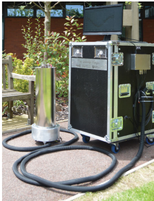
Figure 4. Portable gravity sensor developed at the University of Birmingham as part of the DSTL Gravity Imager programme. (Online version in colour.)
