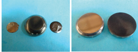
Figure A1. The photos of the ingot with cut off upper and lower “caps” before (left) and after (right) cutting into two halves which served as billets for the fabrication of mirror samples.
