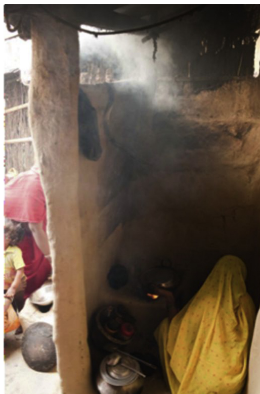
Fig. 1. Typical study kitchen in Janakpur showing cooking stove (single pothole) located in the corner, open entrance door and eaves gap above the stove. The household member (mother) is performing cooking activities (evening meal preparation).
