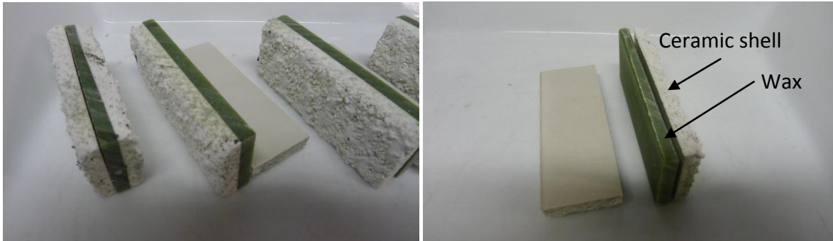
Figure 1- Fridge de-waxing: the shelled flat bar wax was cut after drying to the required test bar dimensions and then separated by cooling in a fridge. The picture on the right shows how clean the ceramic bars are after the de-wax process.
