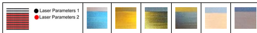
Fig.8. One field coded with two colours using two different laser parameter settings, captured with different incident and azimuthal angles
