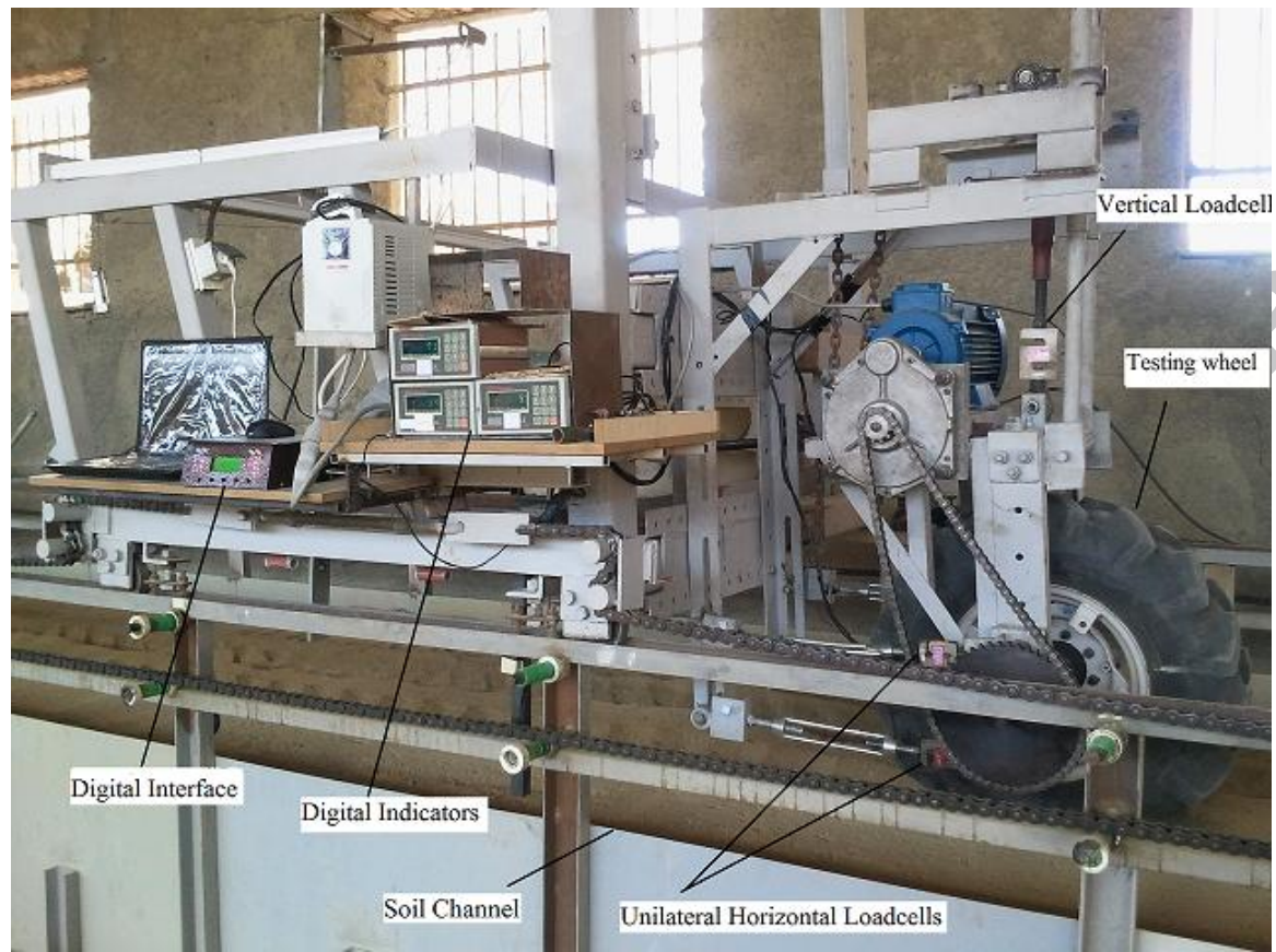
Figure 2- Soil bin testing facility and the components
