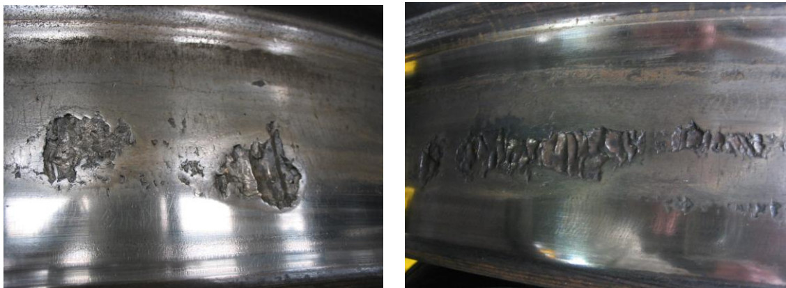
Figure 6: Photographs showing shelling on the tread of the damaged wheel of the EMU tested.
