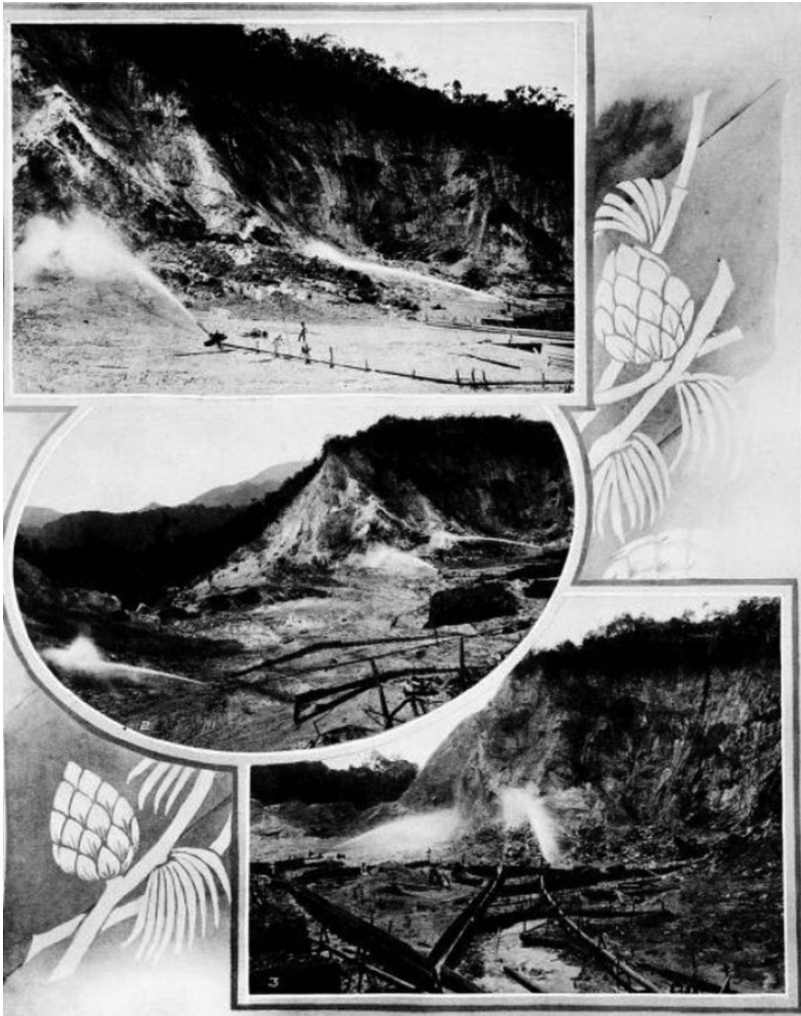
Figure 2: Cutting a 320-foot face at the Bruseh Hydraulic Tin Mining Company, ca. 1908. Arnold Wright and H. A. Cartwright, eds., Twentieth-Century Impressions of British Malaya: Its History, People, Commerce, Industries, and Resources (London: Lloyds, 1908).
