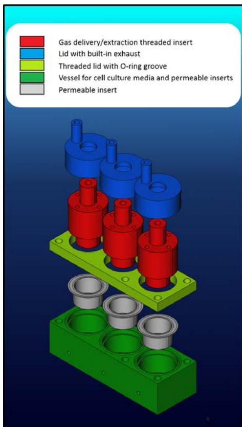
100 Figure 1a: Exploded representation of the exposure vessel with all the part of the assembly.
