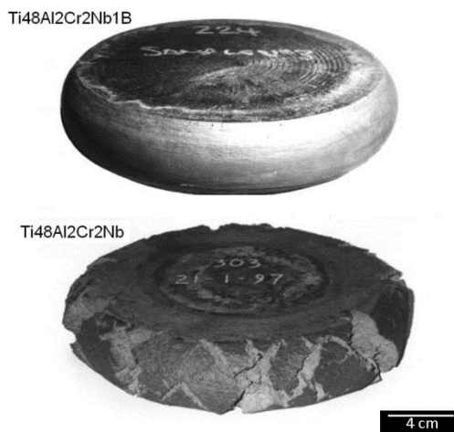
Fig. 14 Surface conditions of Ti48Al2Cr2Nb(1B) after isothermal forging at 1150°C with 70% reduction in height.
