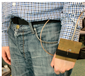
Fig. 2. Monopole antenna on the wrist (2.45 GHz).
