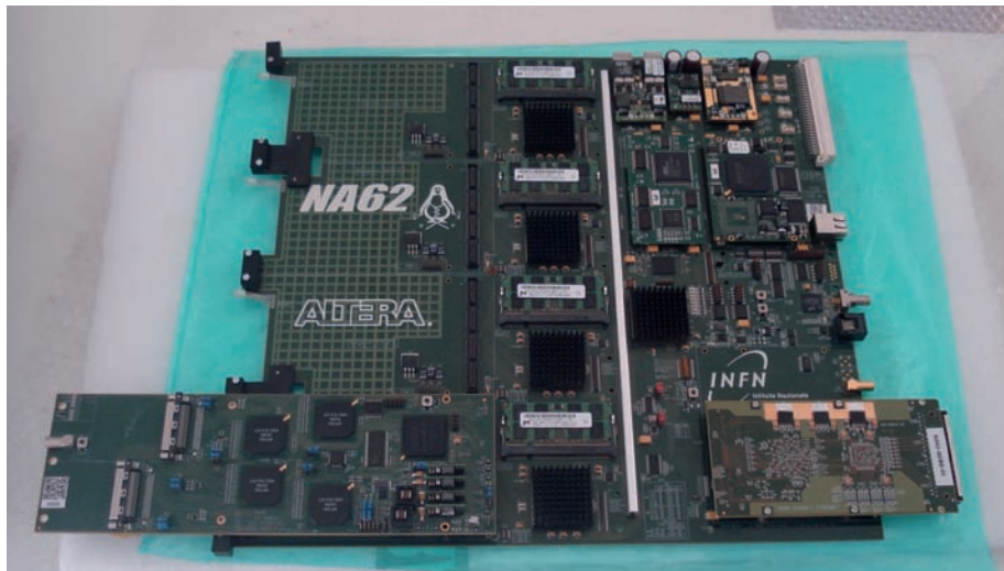
Figure 3: The TEL62 mother board. At the bottom-left a plugged TDCB is also shown.
