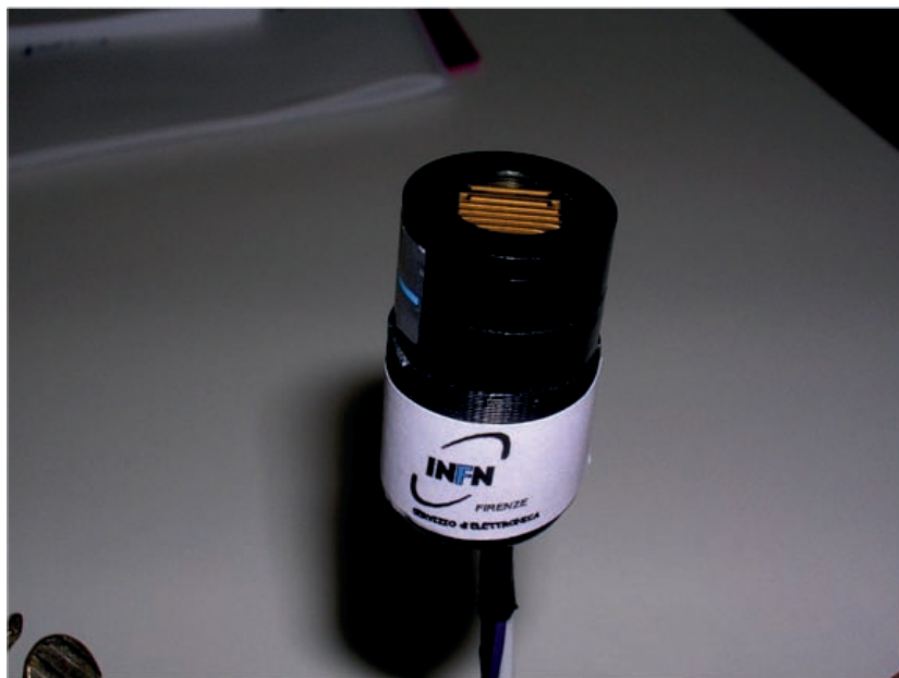
Figure 2: The HAMAMATSU R7400 U-03 photomultiplier connected to the custom made divider.
