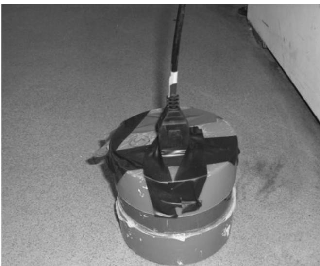
Fig. 2. Completed sample with TDR probe inserted.
