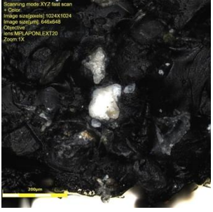
581 Figure 6: From top to bottom, bromine rich particles in dusts 1,2 and 3 respectively: Left – Laser microscopy optical images of particles with 582 measured particle size. Right - SEM backscattering images of particles and related EDS elemental profiles.
