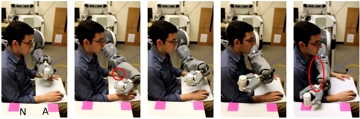
Fig. 9: Image sequence from a trial in the near condition. Contact with the robot indicated in red. Far left: The robot in the starting position, the near goal (N), and away goal, (A).
