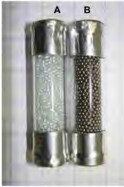
Fig. 14. Cylindrical samples filled with different materials (A: glass spheres, B: stainless steel and \epsilon = 42.5 ).
