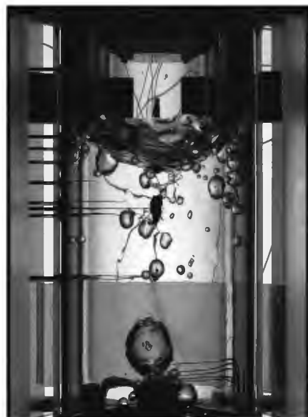
Figure 1: Visualization of pool boiling of HFE7000 in the single species system of SOURCE 2.
