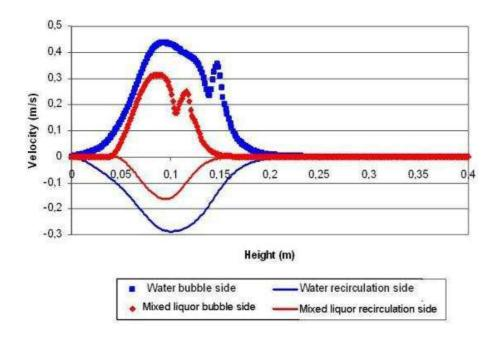
Axial velocities on vertical lines located in the middle of the initialisation of the bubble and at the opposite side of the membrane obtained by CFD
