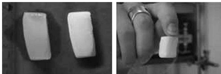
Figure 5. Different gel states of bacterial cellulose obtained from G. xylinum : aquagel vs. aerogel (left). Due to the extremely low density of the material, electrostatic charge is sufficient to make the aerogel stick to a finger (right). Reproduced with permission from Liebner et al. (2010), Copyright Wiley-VCH Verlag GmbH & Co. KGaA.
