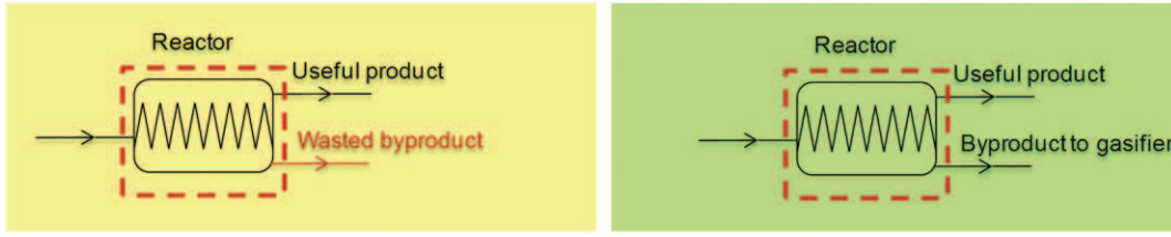
Fig. 9. External exergy loss for a reactor.
