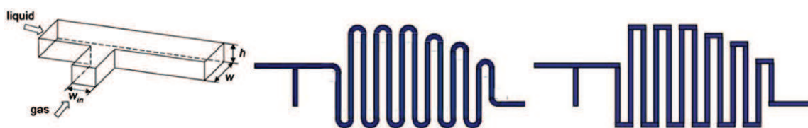
Fig. 1. Schematic diagram of the T-junction microchannel (left) and the topology of the curved (center) and right-angled (right) meandering microchannels.
