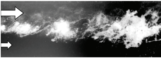
Fig. 2. Instantaneous picture of the cavitating shear layer (Weinberger SpeedCam Visario—shutter time 20 \mu s).
