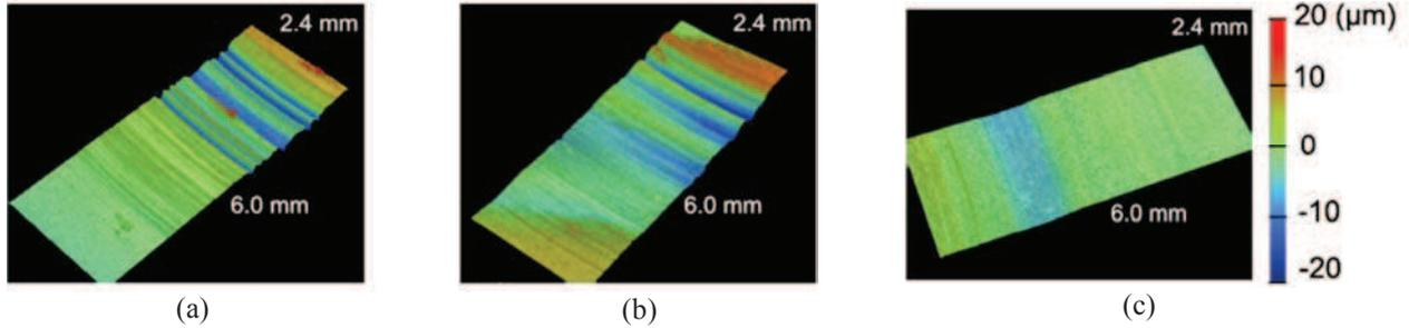
Figure 15: Three-dimensional images of St5WS<sub>2</sub>(a), St10WS<sub>2</sub>(b) and St20WS<sub>2</sub>(c) recorded by profilometry.
