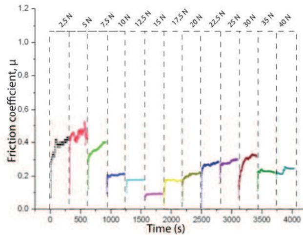
Figure 4: Friction coefficient of St20WS<sub>2</sub> with respect to the time and normal load.
