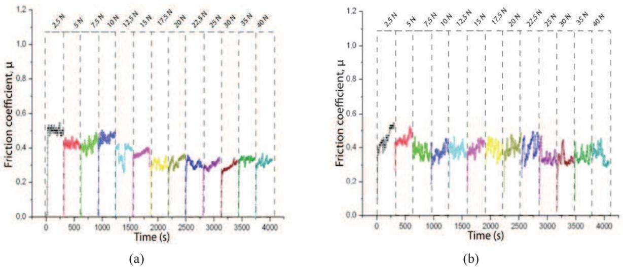
Figure 3: Friction coefficient of St5WS<sub>2</sub> (a) and St10WS<sub>2</sub> (b) with respect to the time and normal load.
