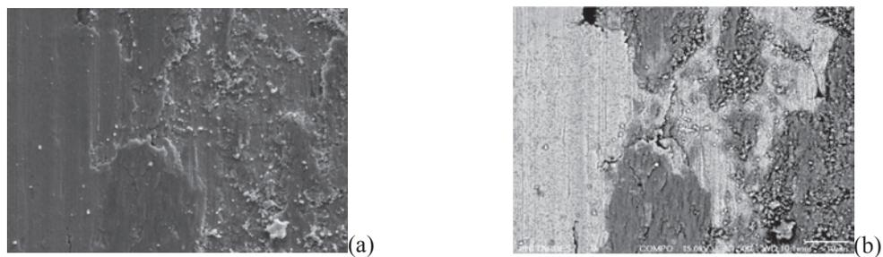
Figure 18: Observations by SEM of the sliding surface of the St10WS<sub>2</sub> with two different observation modes: secondary electron and backscattered electron with chemical contrast.
