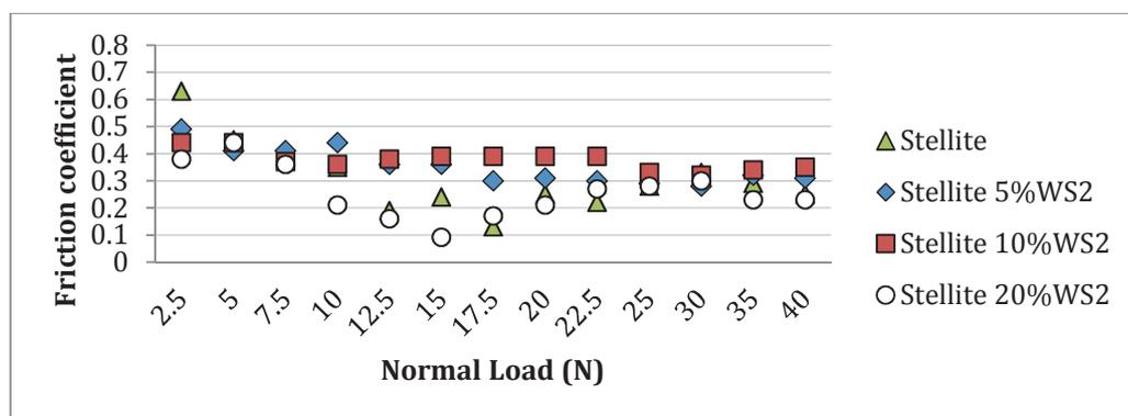
Figure 20: Friction coefficient versus the applied normal load for Stellite, and Stellite with 5%, 10% and 15% (vol.) of WS<sub>2</sub>.
