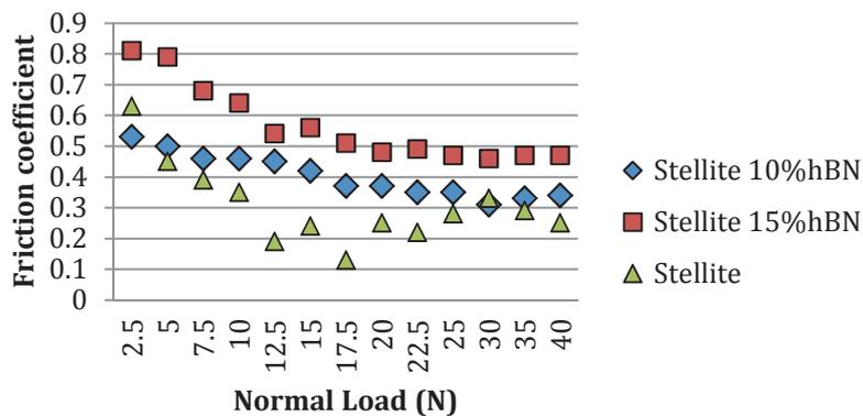
Figure 19: Friction coefficient versus the applied normal load for Stellite, and Stellite with 10% and 15% (vol.) of h-BN
