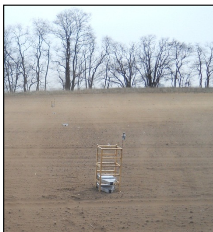
Figure 2. Soil particles catcher disposition during the terrain measurement
