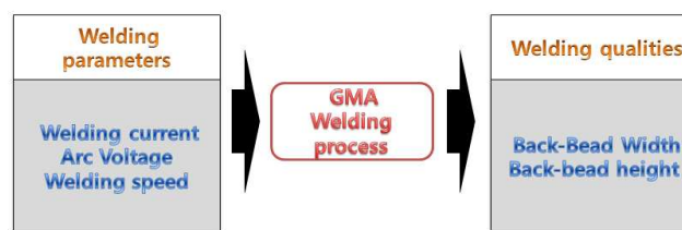
Fig. 1 Analytical algorithm procedure for robotic arc welding
