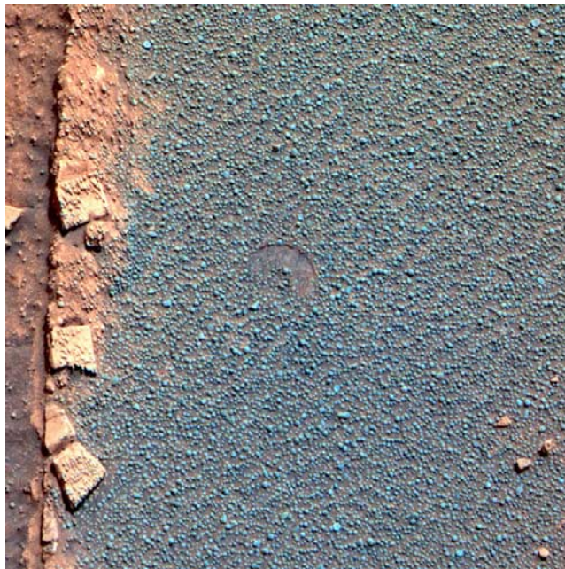
Figure 13. False color Pancam image of disturbed soil near Purgatory Ripple. Reddish indurated clods on the left side of the image have been created by rover wheel interactions with the soil. The partial circular impression near the center of the image was created by the Mössbauer Spectrometer contact plate. Image acquired on Sol 510 using Pancam’s 753 nm, 535 nm, and 432 nm filters, L2, L5, and L7.
