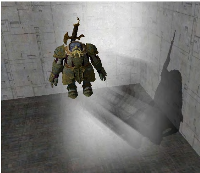
Fig. 4. Initial implementation with external shadowing effect. Artefacts (hard edges) within the 'smoke' are visible.
