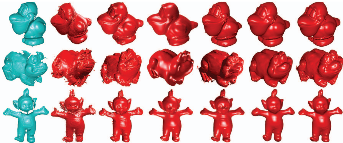
Figure 1. Rows: Reconstructions using 17 Bird range images, 17 Frog range images and 17 Teletubby range images respectively. From left to right: one single range image used as partial ground truth, volumetric method [3], mesh-based method [15], SFK method [20], k-means clustering-based method [19], pairwise MRF-based method [11], higher-order CRF-based method [14]
