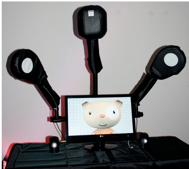
Fig. 5. User's View of the Punchable Interface
