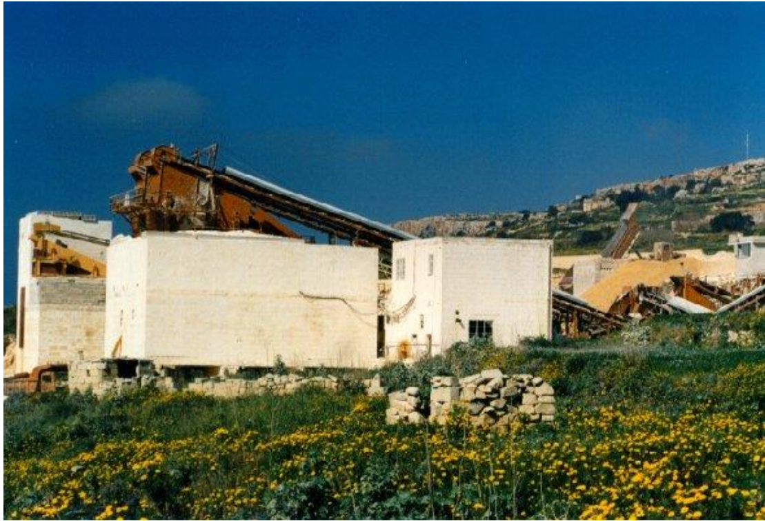
Photo 3: Crushers in a hardstone quarry used to break down rock into required gauge size.
