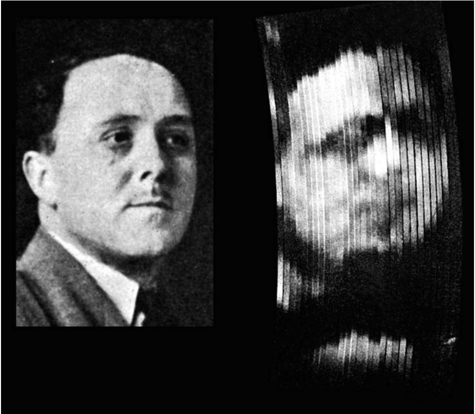
FIGURE 3 Oliver Hutchinson — subject of the earliest photograph of a television image, early 1926. National Media Museum (for image on right).
