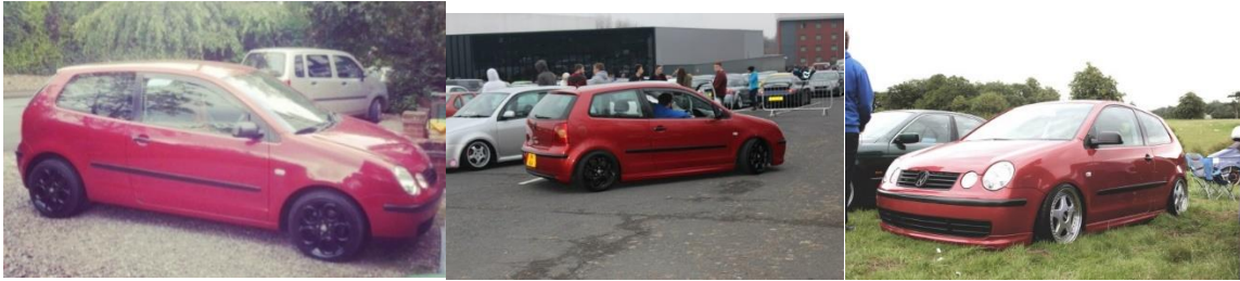
Figure 23. From left to right, my VW Polo with its air suspension in the highest setting, drive height & fully lowered (Author's Photographs).
