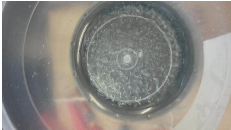
Cymatic experiment with a speaker, bowl and water
