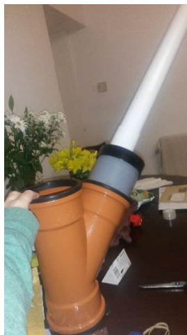
Homemade tonoscope using plumbing fixtures and pipes
