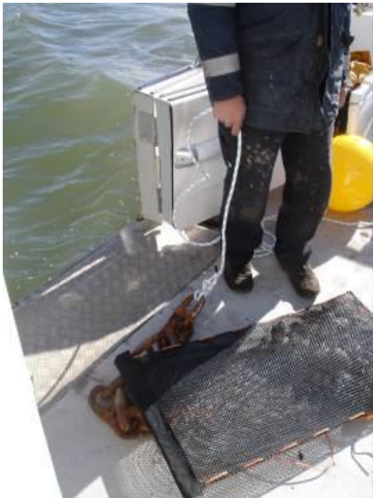
Figure 14 Sampling stations established in the estuary (site 13) showing bag with oysters for sampling (A), mooring chain (B) and mooring buoy (C).
