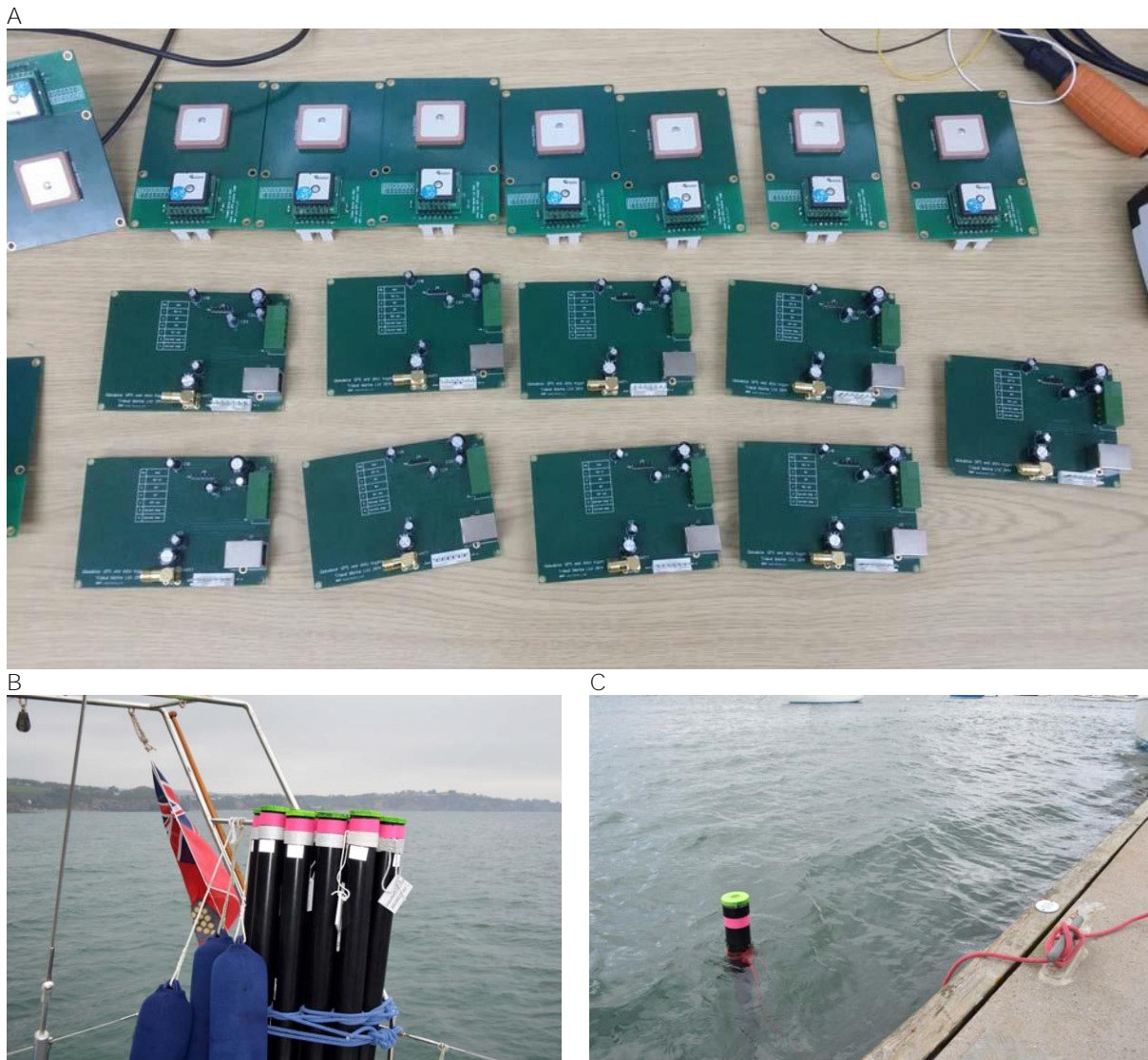
Figure 20 Satellite-tracked drogues used in the bay (site 32) showing electronics prior to building into the drogue casings (A), drogues ready for deployment (B) and ballasted drogue in the water (C).
