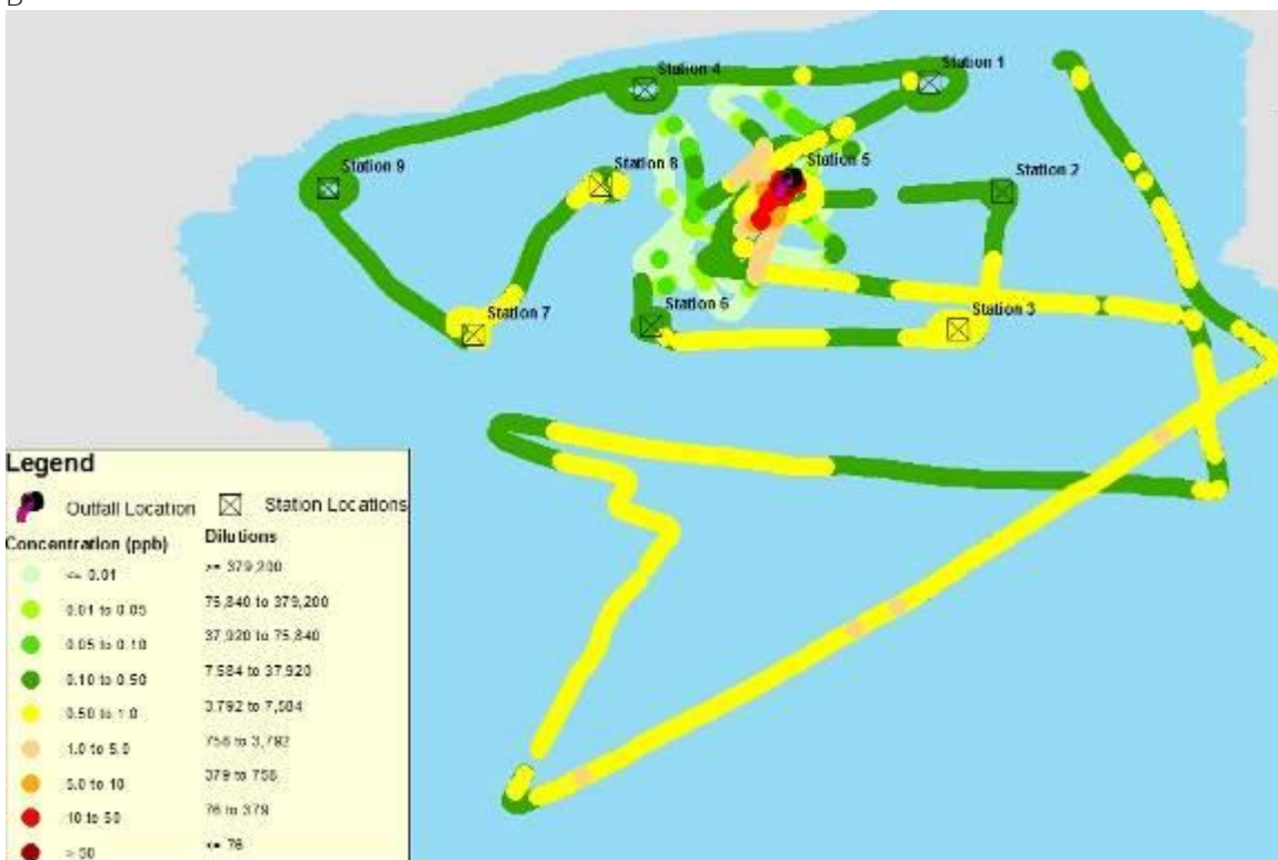
Figure 25 Dye concentrations and dilutions recorded by the towed fluorometers in the estuary (site 13; A) and bay (site 32; B).
