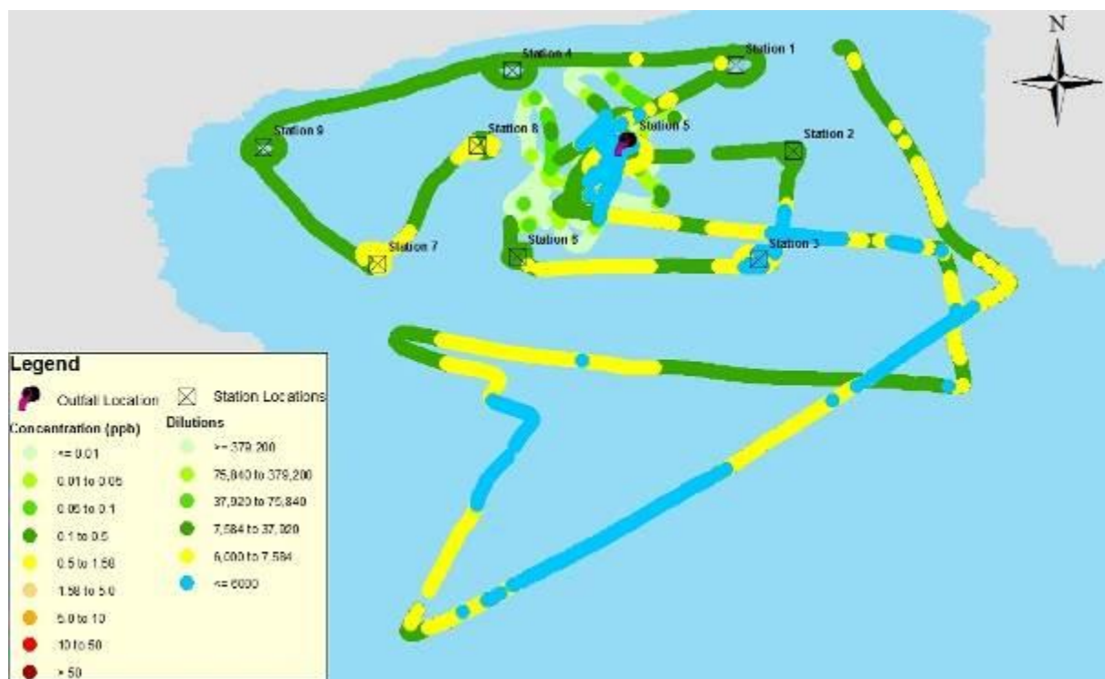
Figure 29 Rhodamine dye concentrations and sewage effluent dilutions recorded by the towed fluorometer in the bay (site 32) on 16–17 June 2015 with dilutions of less than 6,000:1 highlighted in blue.
