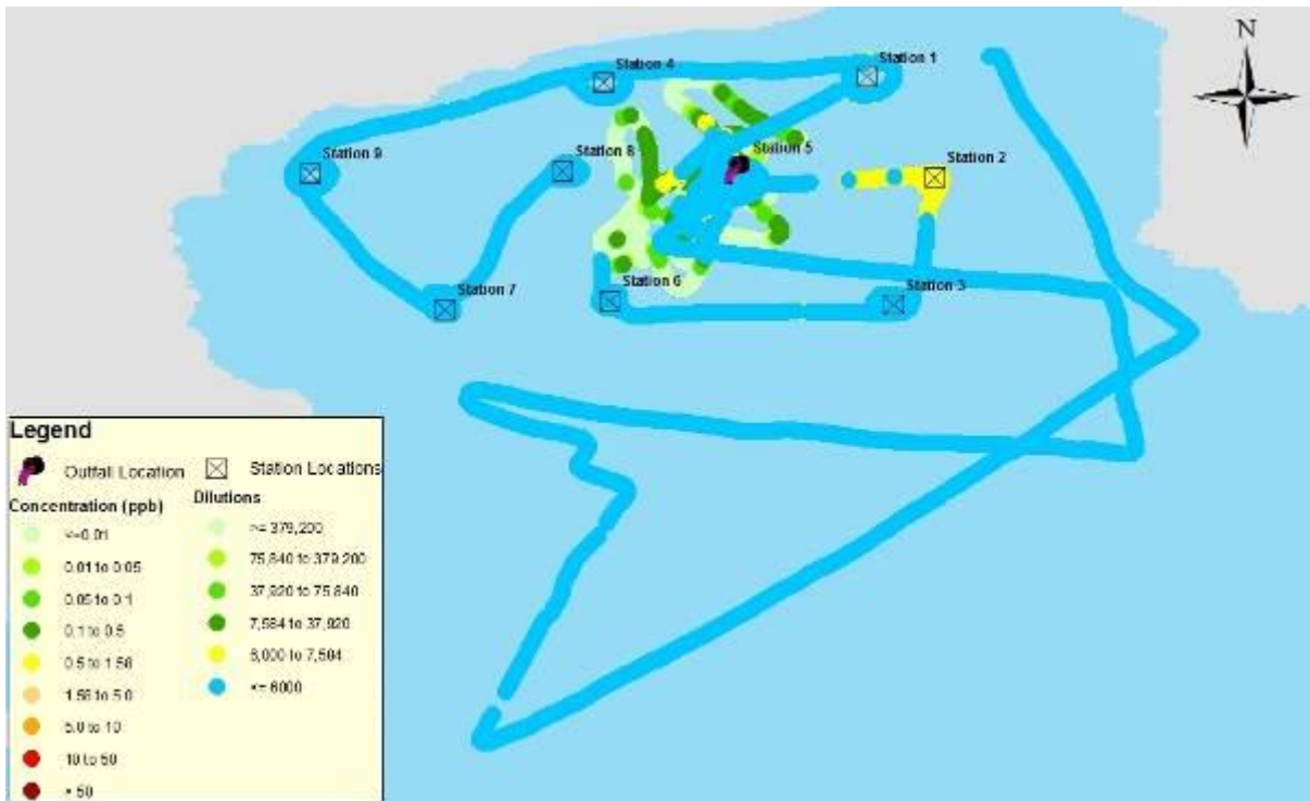
Figure 30 Rhodamine dye concentrations and sewage effluent dilutions recorded by the towed fluorometer in the bay (site 32) on 16–17 June 2015 with dilutions of less than 6,000:1 for the 90 th percentile flows through the STW highlighted in blue.
