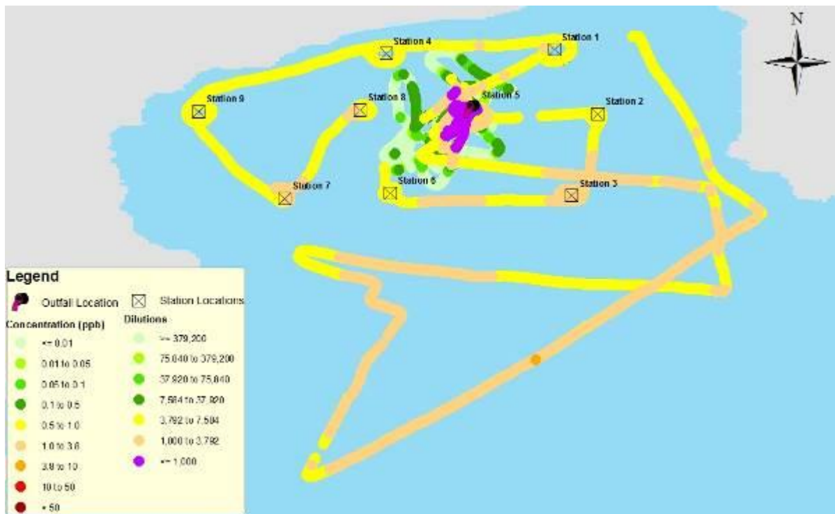
Figure 31 Rhodamine dye concentrations and sewage effluent dilutions recorded by the towed fluorometer in the bay (site 32) on 16–17 June 2015 to illustrate the size of the buffer zone as a result of a new UV disinfection treatment at sewage treatment works D.
