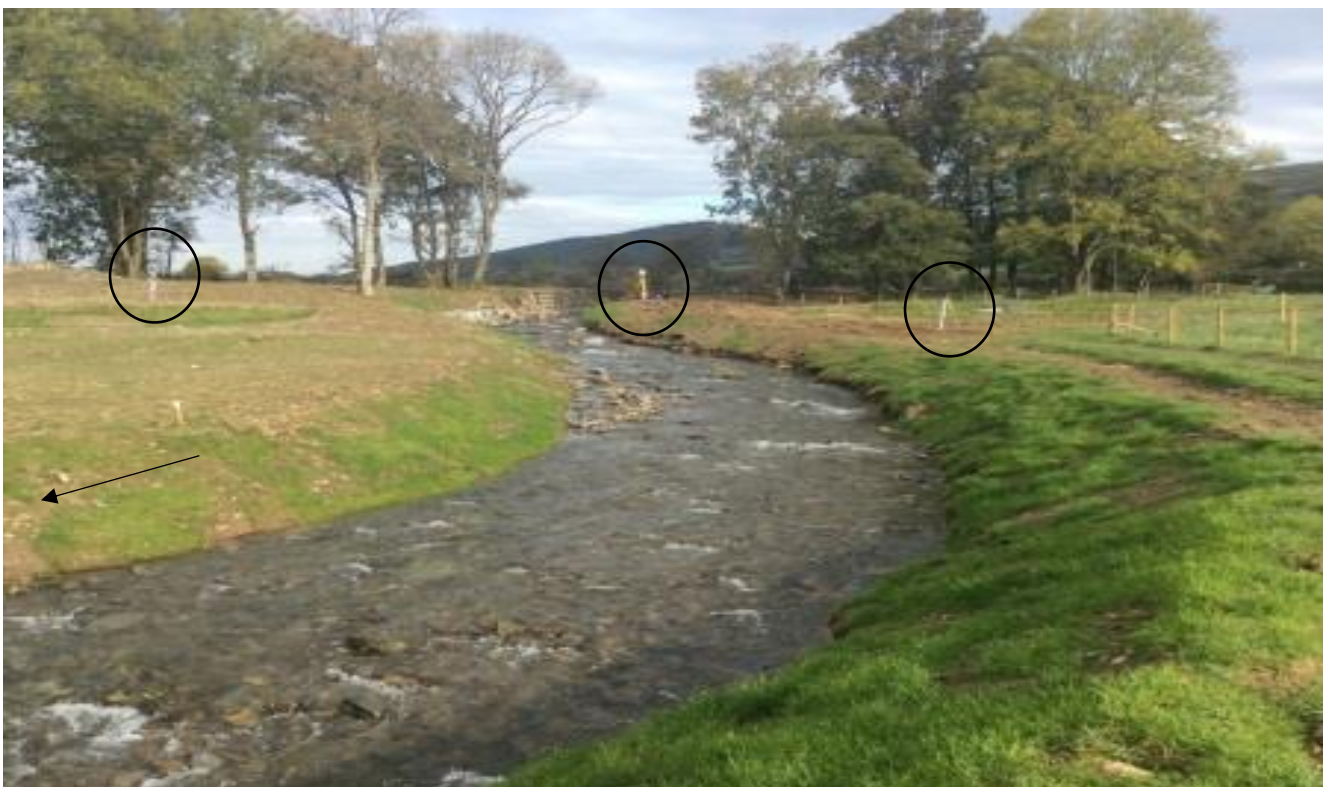
Figure 3.25: Showing how targets are set out when a TLS scan is being carried out to ensure a wide spatial representation. The main scanner is shown in the centre circle, while two targets are shown on the left and right side. The third target was situated 50 m downstream of the arrow on the left side bank (looking upstream).
