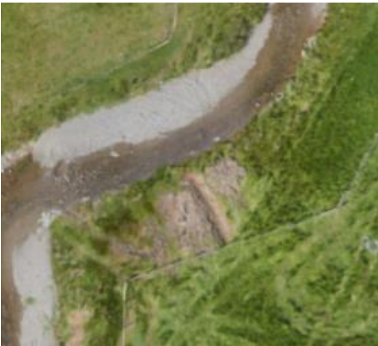
Figure 5.4: DoD change at location A (on Figure 5.1). A. DoD showing areas of erosion and deposition. Bar growth (deposition) and gully formation have been mapped. B. October 2014 orthophoto and c. July 2015 orthophoto to show change in graphical form. River outline shown.
