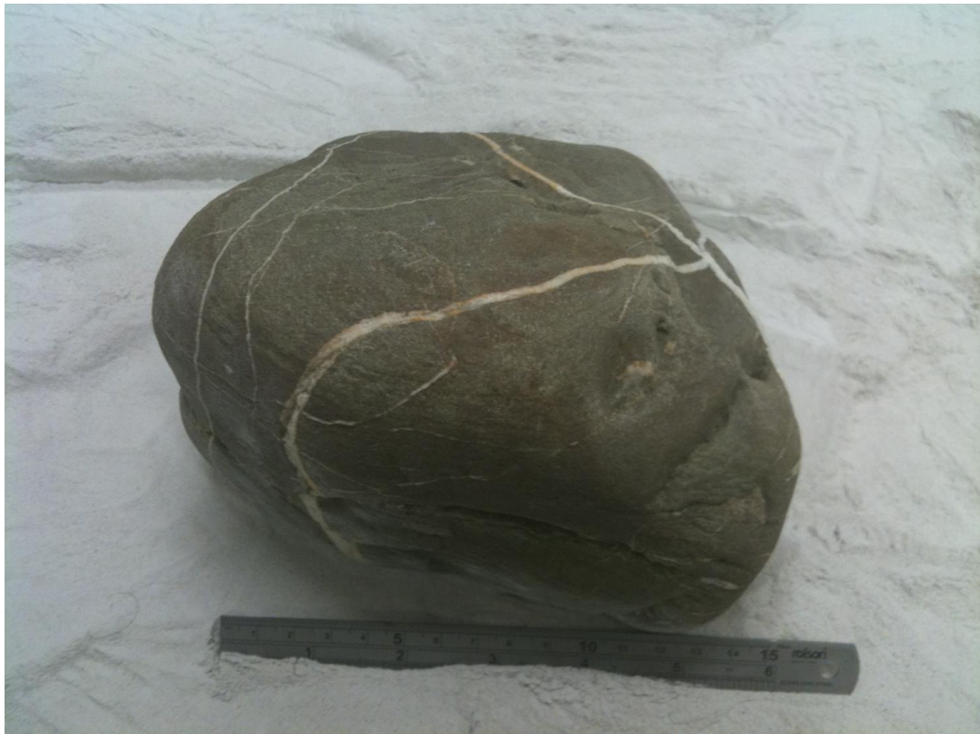
Figure 2.6: Example rock target demonstrating lamination features.
