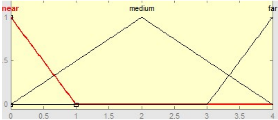
Figure 4.8: Membership functions for the Distance ( i_d ).
