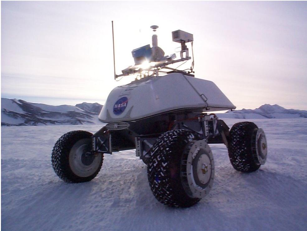
Figure 2.1: Image of Carnegie Mellons Nomad Rover (Image courtesy of Carnegie Mellon). Nomad is a 4 wheel drive rover measuring 2.4 \text{ m} \times 2.4 \text{ m} \times 2.4 \text{ m} , and has a total mass of just over 700 kg
