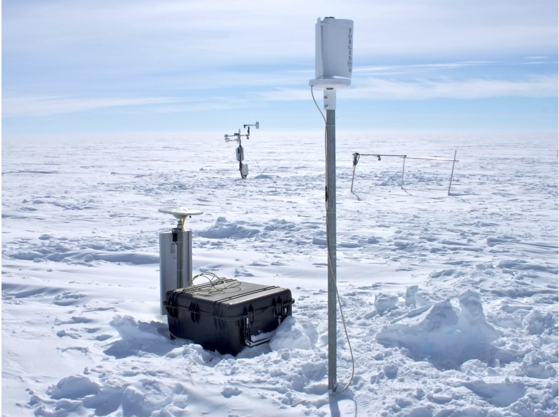
Figure 7.1: Photo of the GPS installation at S10. In the background is the KAN_U weather station (left) and stake assembly (right). 4 May 2012.
