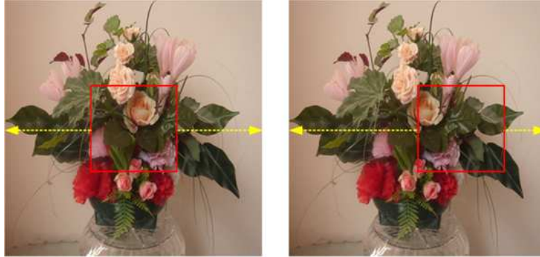
Figure 4.33 – Locating the patch in the most central position gives equal tracking opportunity to both sides
