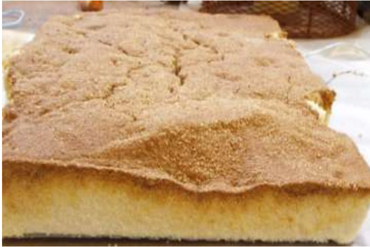
Figure 7.19. Sand bed from the 1 L/minute Esgair Hir treatment plant after 15 days.
