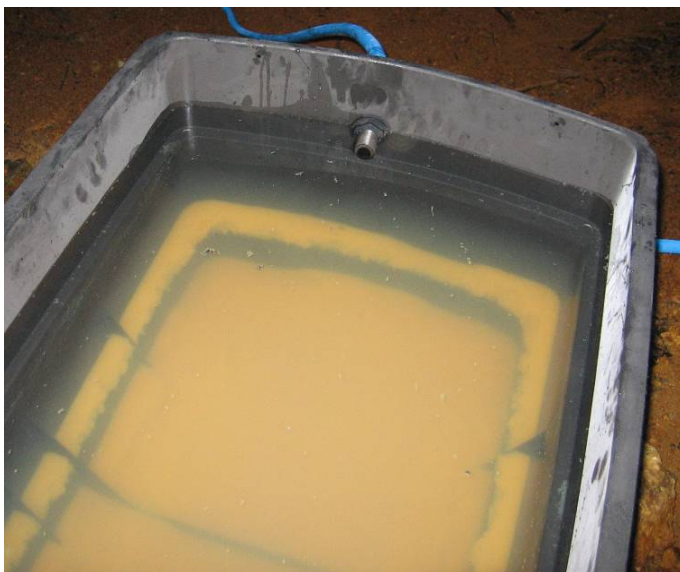
Figure 8.11. Settlement of the formed flocculates.
