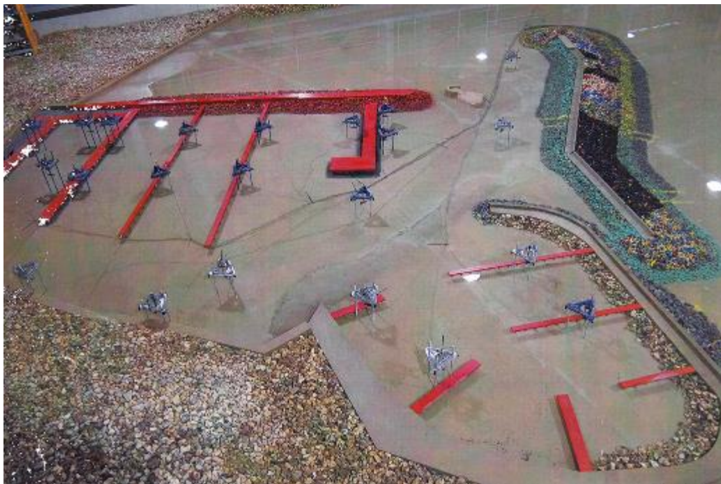
Figure 8. Model for studying harbour designs. Source: R. Raviv Consulting Engineers (2013).
