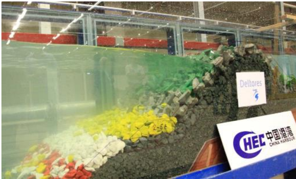
Figure 7. Model for study concerning designs of an offshore breakwater. The model is located in a ‘wave flume’. Source: Coasts, Deltas and Rivers International (2014).
