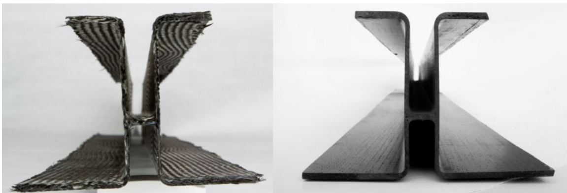
Figure 2-21 Near-net Shape Fabric (Left) and Net Shape Composite (Right) [42]
