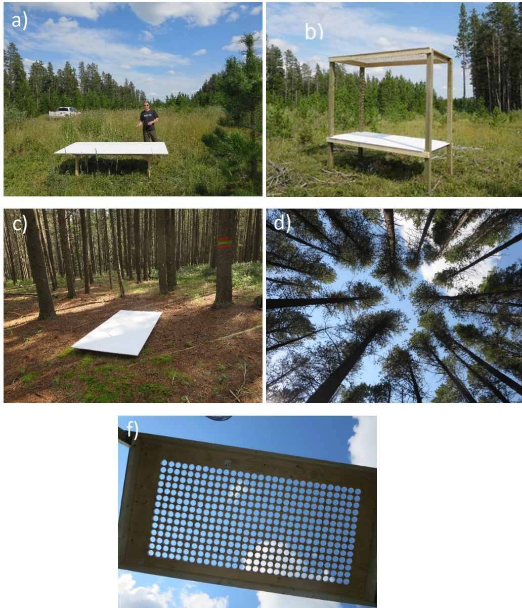
Figure 4.1 Photos of the radiometric calibration targets (made from 8' by 4' plywood). Photos a), b), and c) – are an open target, lifted target, and below-canopy target, respectively. Photos d) and f) illustrate corresponding transparency of the Lodgepole Pine foliage above the target and transparency of the lifted target.
