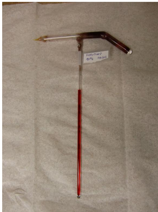
Figure 6.3. “T” cell for chemical oxidation EPR experiment containing \text{AgPF}_6 and \text{Tripp}_2\text{DippP}
