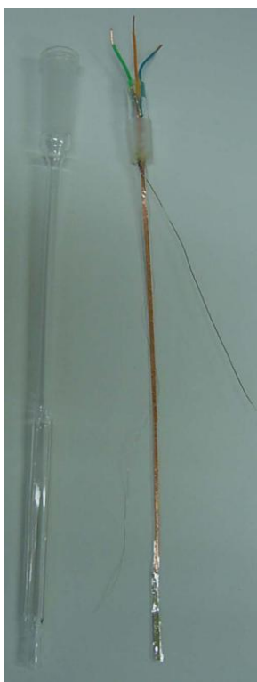
Figure 2.6. Low-temperature EPR flat cell developed by Boéré and Roemmele
