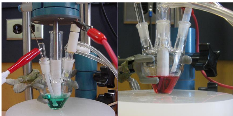
Figure 6.1. RDE cell containing [\text{Dipp}_4\text{P}_2]^{+/0} (blue solution) and [\text{Dipp}_3\text{As}]^{+/0} (red solution)
