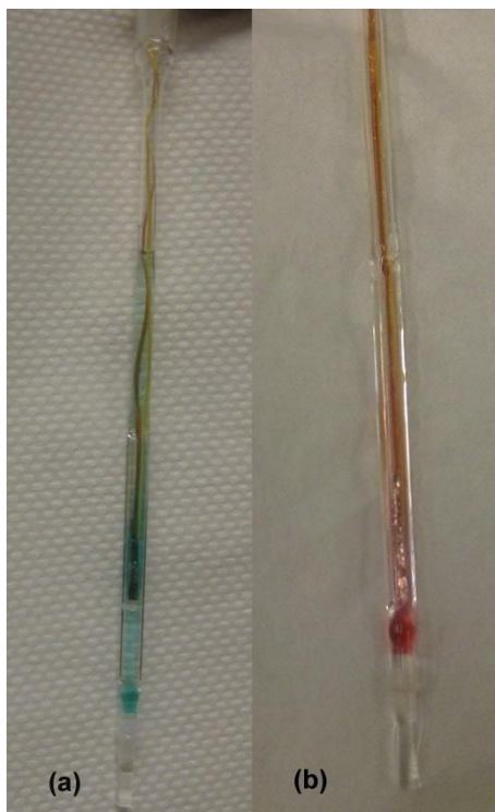
Figure 6.2. SEEPR cell containing (a) [\text{Dipp}_4\text{P}_2]^{++} and (b) [\text{Tripp}_2\text{DippP}]^{++}
