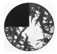
Figure 3.5 : Fisheye photo as viewed by the LAI-2000 fixed with a  $270^{\circ}$  lens attachment (Licor, 2010). The  $270^{\circ}$  lens attachment allows light to enter the lens at  $270^{\circ}$  and blocks light into the remaining  $90^{\circ}$  (dark region). Figure taken from Licor (2010), and does not correspond to any crop type, DAP or wavelength related to this study.
