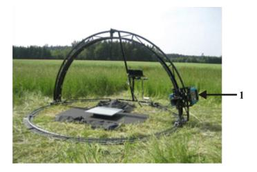
Figure 2.3 : The FIGOS field goniometer assembled with the GER-3700 spectrometer (1) (Sandmeier and Itten, 1999). Note damage to target by the azimuth rail.
