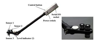
Figure 2.13 : The TRAC instrument (Leblanc et al., 2002). Sensors 1 and 2 measure the DW total diffuse PAR through the canopy and Sensor 3 measures the PAR reflected from the ground.
