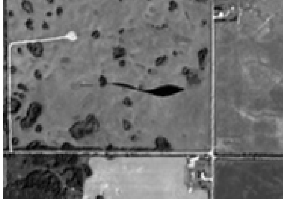
Figure 4.3: After the flight lines were mosaicked an area of no data due to insufficient flight-line overlap was discovered, shown as the black area in the middle.
