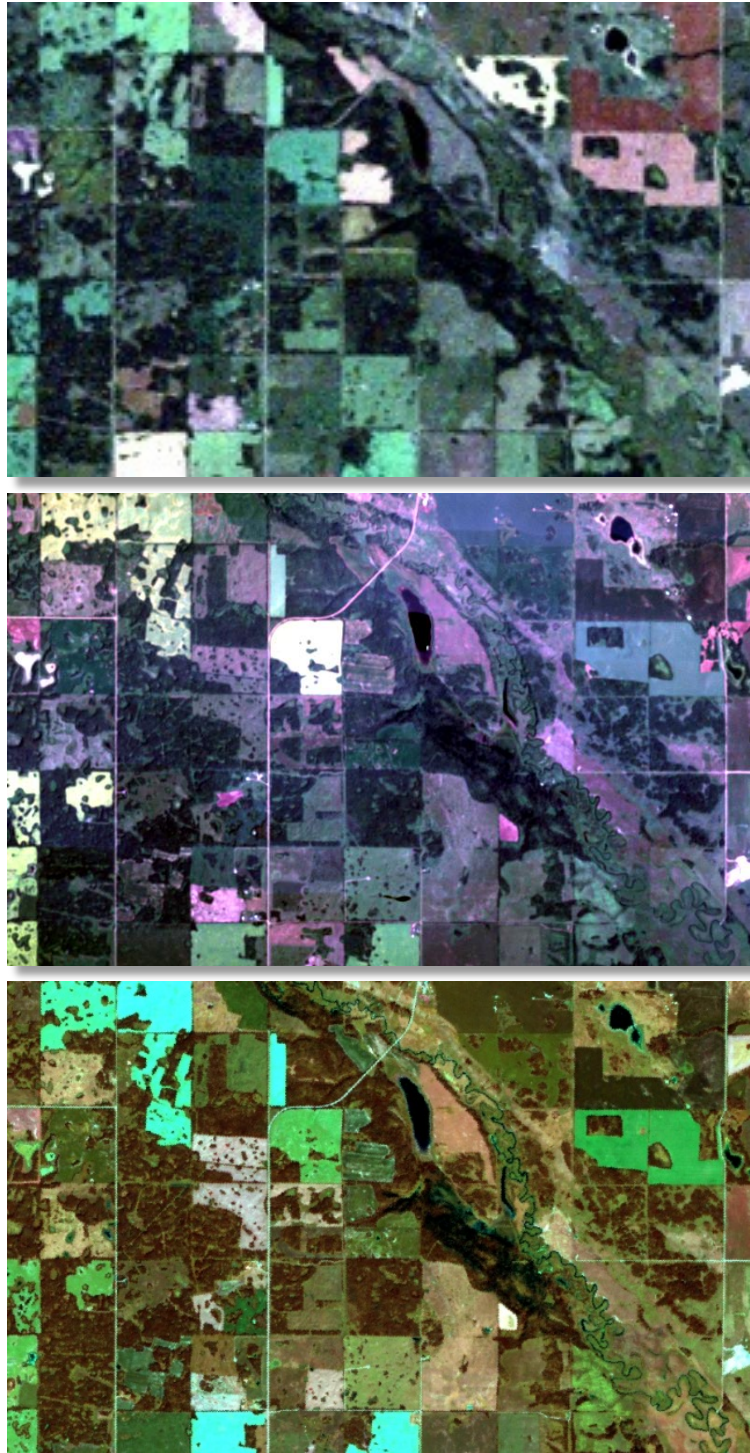
Figure 3.4: True-colour Landsat TM (top) R: Band 3 G: Band 2 B: Band 1, Simulated Sentinel-2 MSI (middle) R: Band 4 G: Band 3 B: Band 2, and Natural-colour SPOT HRV image R: Band 2 G: 0.75B1+0.25B3 and B: 0.75B1+0.25B3 (bottom).
