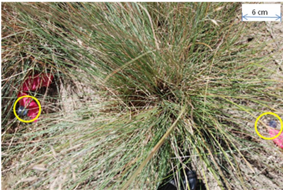
Figure 2.11: Photo of sample containing reference marks of spike heads (circled) to the left and right of the sample marked with strips of surveyor's tape.
