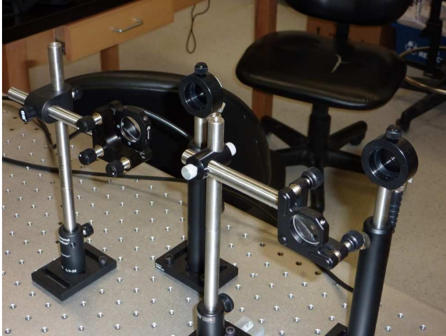
Figure 3-9: Image of two of the three InGaAs detectors used to measure the signals for the tunable diode laser spectrometer. The detectors can be seen just opposite the focusing lenses.
