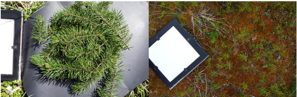
Figure 12: Optically thick stack of jack pine branches (left) and the area of an integrated measurement of orange moss and Labrador tea (right). Spectralon panel included for reference.
