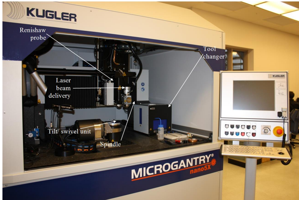
Figure 3. The modular, multi-functional micromachining system Microgantry nano5X and its components.
