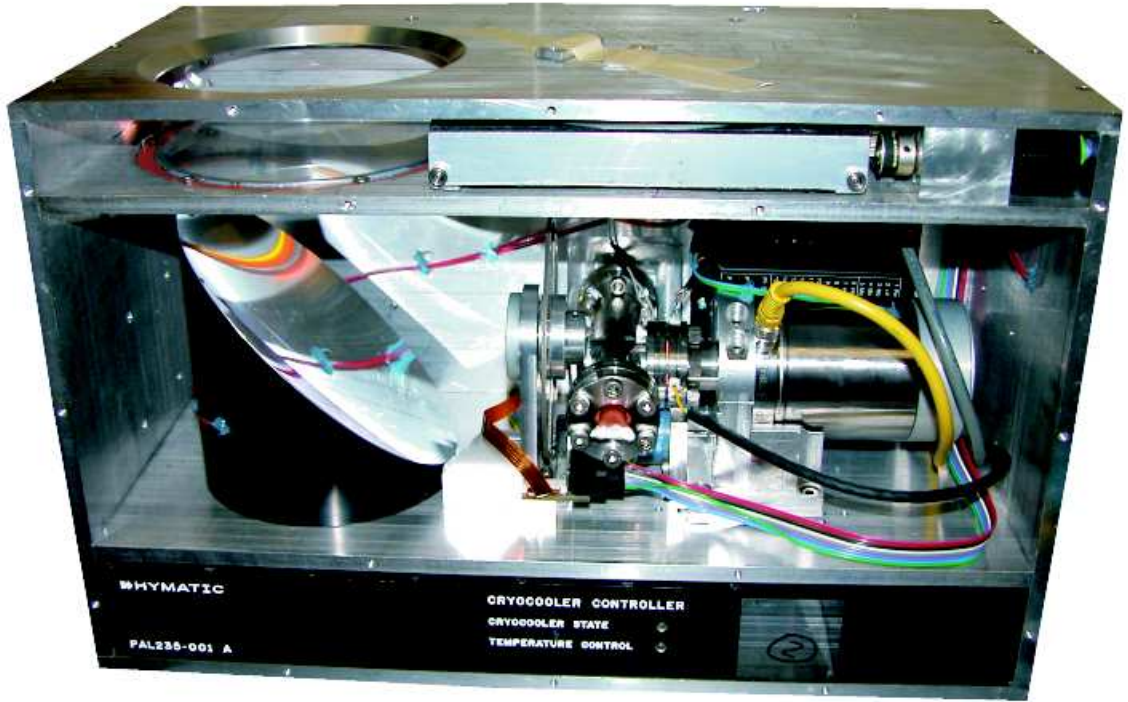
Figure 6.2: Photo of the optical side of the IRMA instrument. The shutter/internal blackbody is open. Components including the detector assembly, the cooler controller, chopper wheel, and paraboloid mirror can be seen from this side of the unit. The far side (not pictured) houses the electronics.
