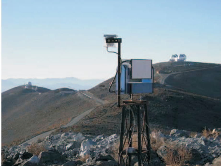
Figure 6.3: An IRMA unit installed at the Las Campanas Observatory. The Magellan telescopes are shown in the background (right).
